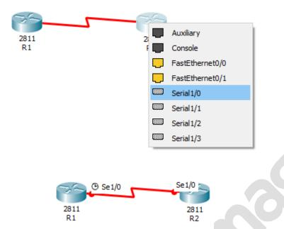
7. Click on the Router R1 and select the CLI (Command Line Interface) tab and enter the following commands. Type "no" or "n" when asked if you would like to enter the initial configuration dialog and press Enter twice.
