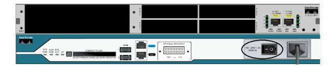
4. Under the Modules, click on the 4-port asynchronous/synchronous serial network module (NM-4A/S) from the list and drag and drop it onto the Router slot as shown in the figure below and then switch the Router back on by pressing the Rocker Switch once.
