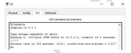
15. Check the Router's Configuration via the Command Line Interface.
