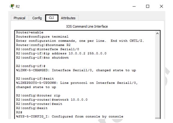
12. Click on the Router R2 and select the "Config" tab to verify the Router's Configuration Settings as in steps 8, 9 and 10 for the Router R1.
