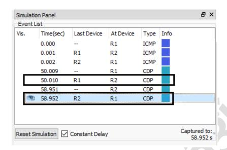
18. Observe the PDU Information at the Device by clicking on the CDP event in the Event List. Under the OSI Model Tab view the "In Layers" model. Click on the Next Layer Button to observe the processes taking place at each layer of an event. Under the Inbound PDU Details tab you may observe the PDU Formats i.e. (High-Level Data Link Control) HDLC, CDP, CDP TLV (Type Length Values).
