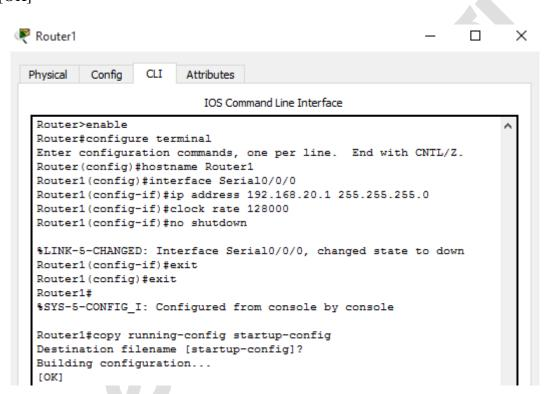
7. Click on the Router1 and select the "Config" tab. Under the Serial 0/0/0 Interface tab, verify the configuration settings.
