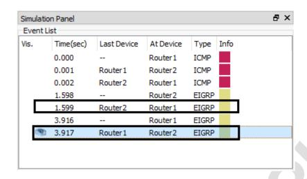
17. Observe the PDU Information at the Device by clicking on the EIGRP event in the Event List. Under the OSI Model Tab view the "In Layers" model. Click on the Next Layer Button to observe the processes taking place at each layer of an event. Under the Inbound PDU Details tab you may observe the PDU Formats i.e. (High-Level Data Link Control) HDLC, IP, EIGRP, EIGRP Parameters, EIGRP Software Version.
