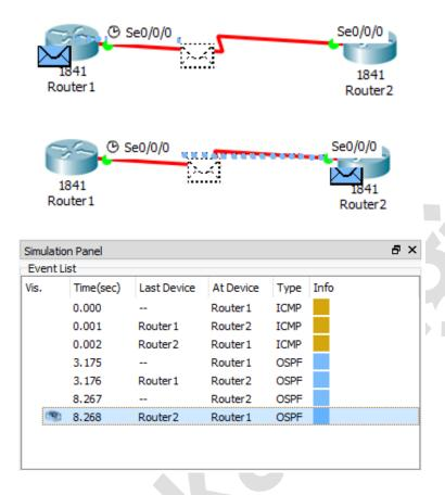
15. Observe the PDU Information at the Device by clicking on the OSPF event in the Event List. Under the OSI Model Tab view the "In Layers" model. Click on the Next Layer Button to observe the processes taking place at each layer of an event. Under the Inbound PDU Details tab you may observe the PDU Formats i.e. (High-Level Data Link Control) HDLC, IP, OSPF Hello.
