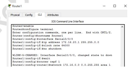
7. Click on the Router1 and select the "Config" tab. Under the Serial 0/0/0 Interface tab, verify the configuration settings.
