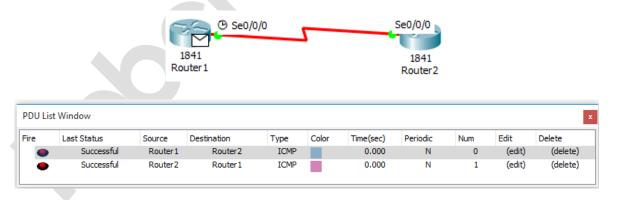
14. Press Ctrl+Shift+D to Delete the Scenario and all PDUs. Press Shift+S to enter into the Simulation Mode. Press "P" to Add a Simple PDU. Click on the Router1 then click on the Router2. Press Alt+C or on the Simulation Panel under the Play Controls click on the Capture/Forward button multiple times until you observe successful implementation of the OSPF under the Event List on the Type Column.
