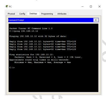
22. Perform a ping command to check the connection between the PC and Router by pinging it with the Router's IP Address (192.168.10.1).
