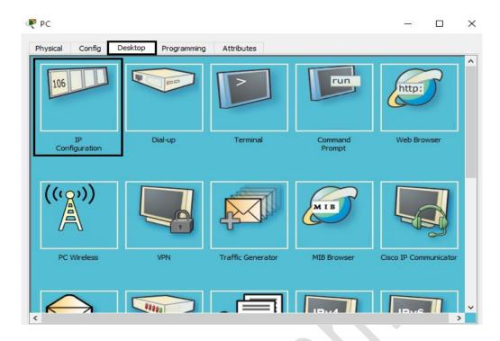
16. In the IP Configuration of the PC, select the DHCP radio button and wait for the PC to complete the request for its IP address from the DHCP Router. Notice that the ip addresses ranging from 192.168.10.1 to 192.168.10.10 are excluded as per the given commands in step 12.
