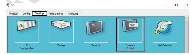
21. Perform a ping command to check the connection between the PC and printer by pinging the PC with the DHCP given address of the Printer (192.168.10.12).
