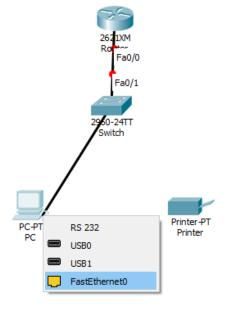
9. Select the copper straight- through cable again, then click on the Switch once more and select the FastEthernet0/3 interface.
