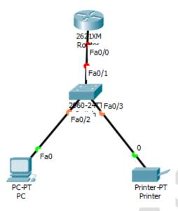
12. Click on the 2621XM Router and select the CLI (Command Line Interface) tab and enter the following commands. Type "no" or "n" when asked if you would like to enter the initial configuration dialog and press Enter twice.
