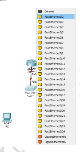
8. Next, click on the PC and select the FastEthernet0 interface to complete the connection between the Switch and PC.
